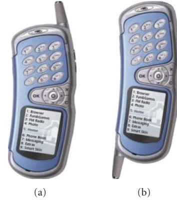
FIGURE 1: The physical model of (a) the handset released by Linux, and (b) the proposed handset with bottom-mounted antenna.
