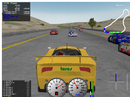
Fig. 1. A screenshot during a test of a previously trained driver. The driver receives 180.000 inputs ( 600 \times 300 ) one from each pixel from the viewport in front.
