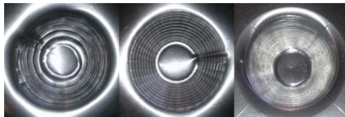
Figure 7.8: Truncated cones made using 10, 5 and 1 millimetre vertical increments.
