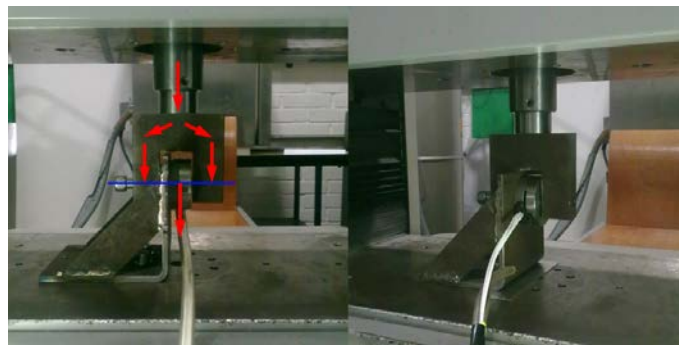
Figure 3.19: Shear load testing mechanism.
