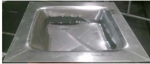
Figure 7.6: Ruptured part while attempting 70° wall.
