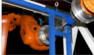
Figure 2.20: Serial industrial manipulator performing SPIF operations [41].
