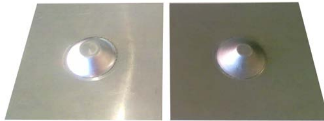
Figure 7.11: Truncated cones made from aluminium and dual phase steel.
