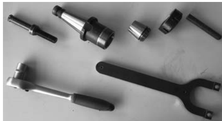
Figure 3.11: Tool holder components (top) and clamping tools (bottom).
