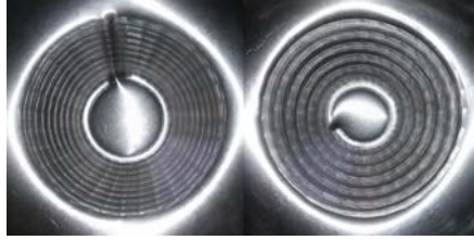
Figure 7.9: Parts made using contour milling and spiralling paths.
