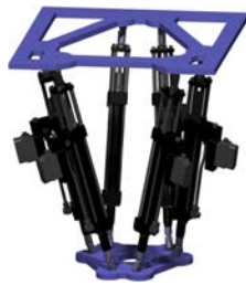
Figure 3.10: Final design of Stewart platform for the SPIF-A.
