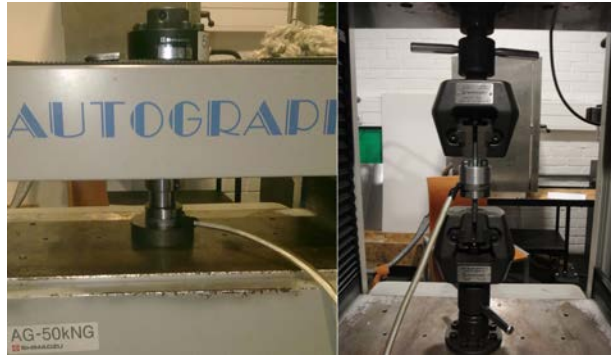
Figure 3.18: Compression and tensile load testing along Z-axis.
