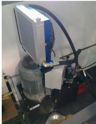
Figure 3.25: SPIF-A's hydraulic pump and heat exchanger installation.
