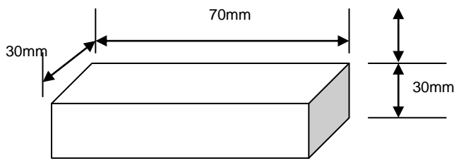
Figure 4: Rectangular box bolted to the bottom of the hopper
