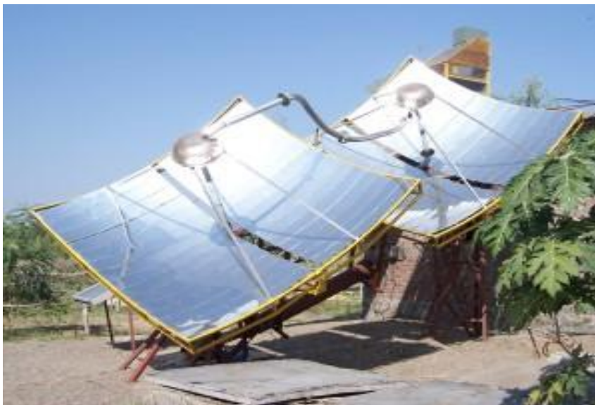
Figure 2.10: Parabolic solar concentrator by Prof. Ajay Chandak
