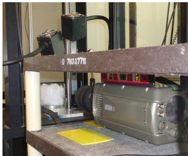
Figure 4.8 High-speed camera used in drop test experiments.
