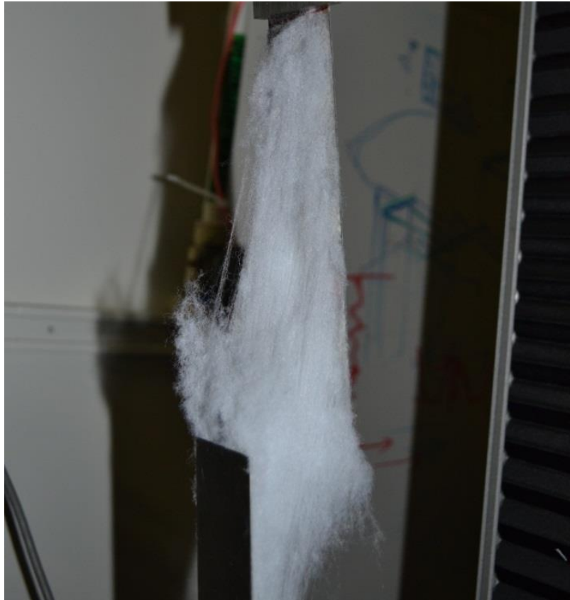
Figure 4.21 Shear specimen 005 near end of test.
