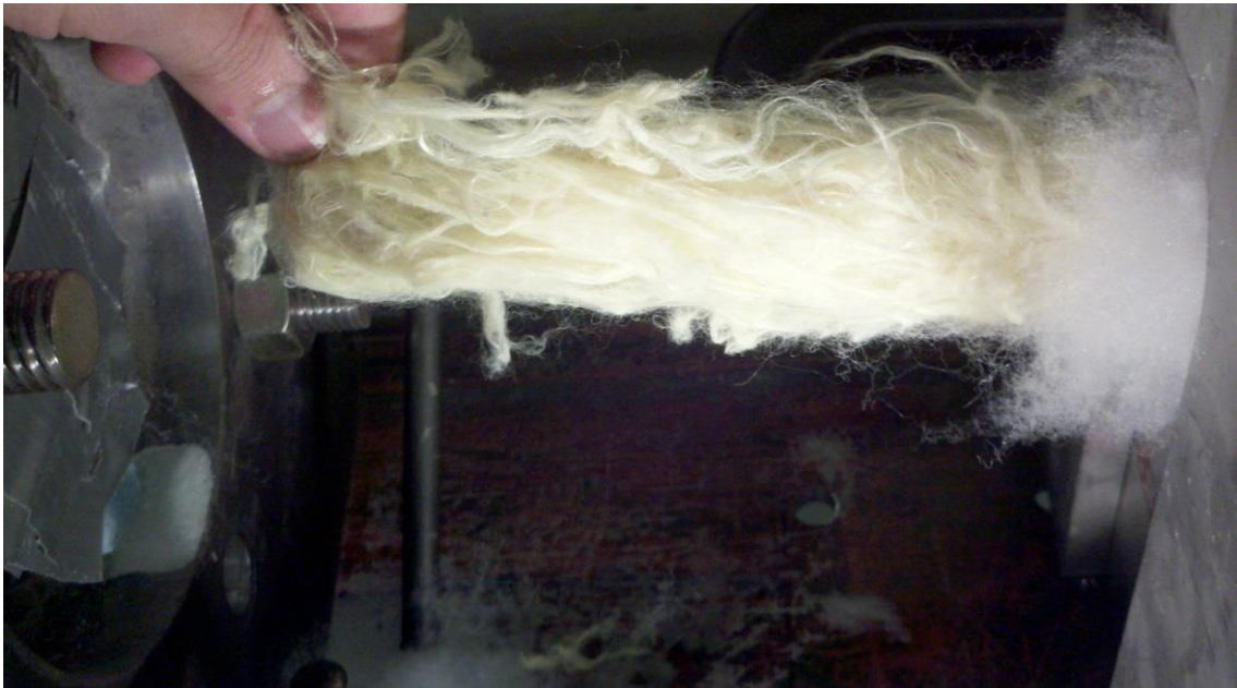
Figure 5.14 Projectile stopped in a Kevlar tail
