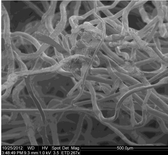
Figure 3.6 Fibers from the projectile affected region showing melting and adhesion.
