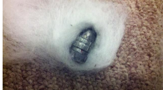
Figure 3.3 Defeated projectile being extracted from a “cocoon.” The tail on this projectile has already been removed.
