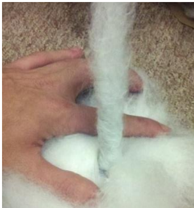
Figure 3.4 "Tail" structure following projectile path.
