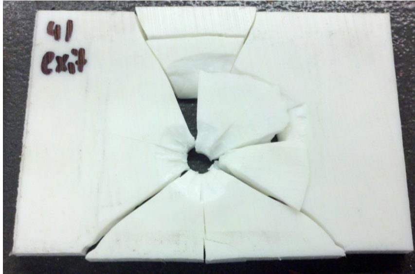
Figure 5.12 PET specimen showing cone and radial cracking after being impacted at 293 m/s
