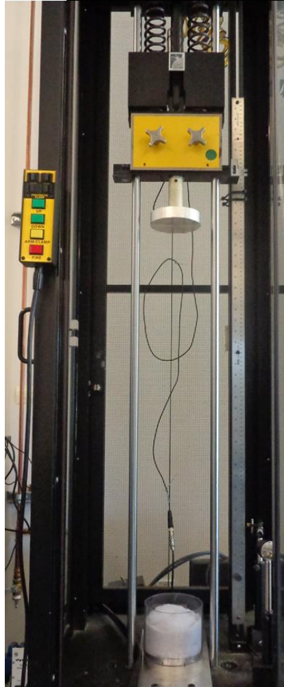
Figure 4.7 Drop test fixture mounted in the Dynatup drop tower.
