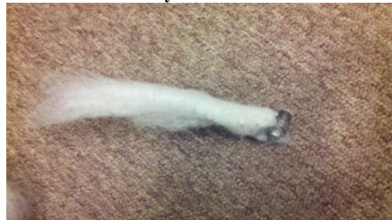
Figure 3.5 "Tail" emanating from the side of a defeated projectile.
