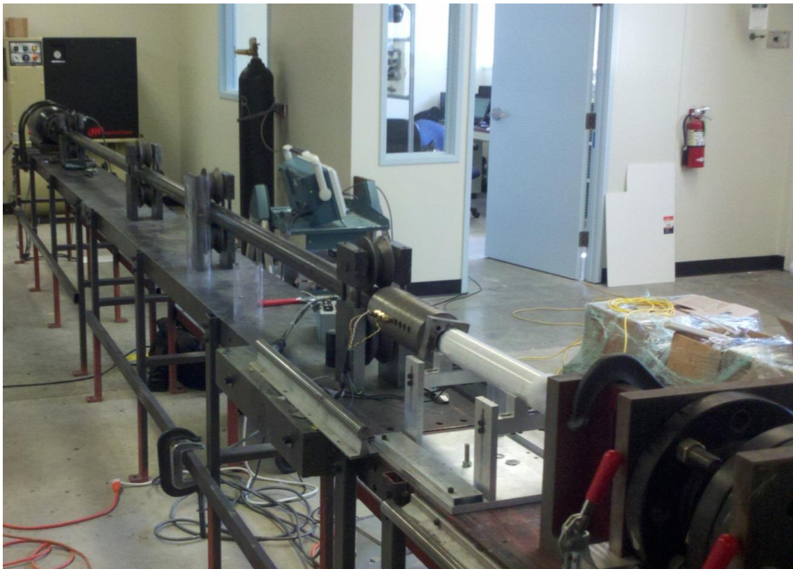
Figure 5.1 Gas gun configured with 45 mm barrel
