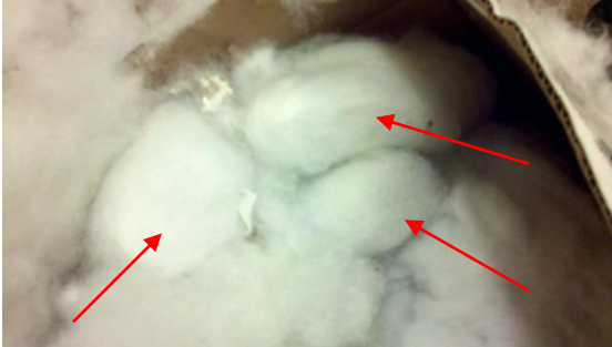
Figure 3.2 "Cocoon" structures surrounding defeated projectiles.
