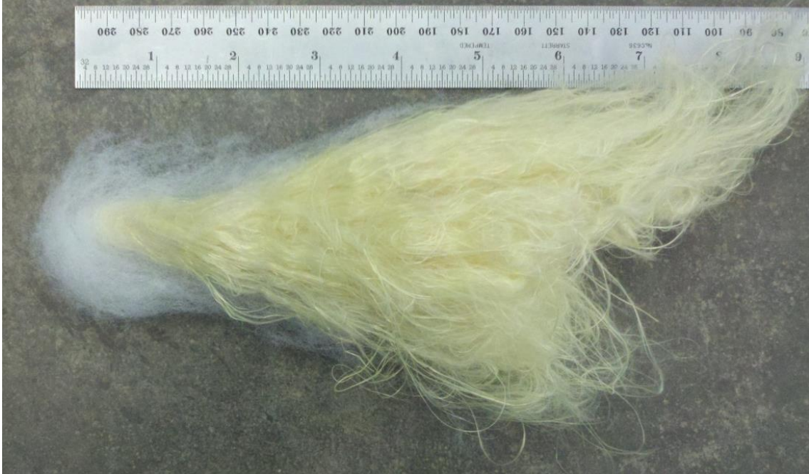
Figure 5.13 Kevlar/PET fiberfill enveloping a defeated projectile
