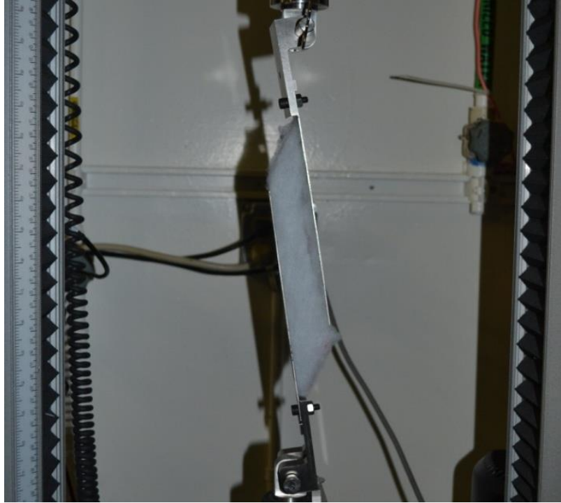
Figure 4.20 Shear specimen 005 at 100% shear strain.
