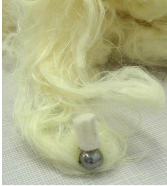
Figure 5.15 Defeated projectile with foam obturator still intact
