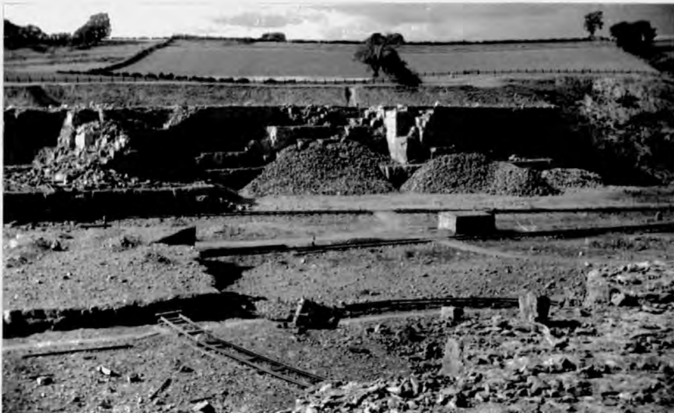
B. Jointing in a small part of East Layton quarry. Three principal directions can be seen.
