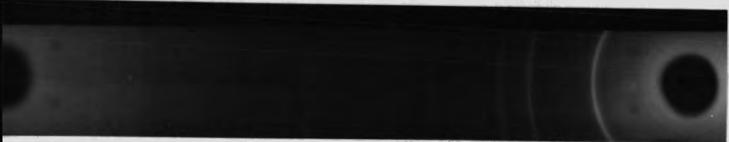
FIGURE 6.4.7 X-ray diffraction photograph of milled (cubic) CdSe
