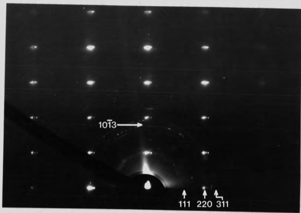
FIGURE 6.5.4 RHEED pattern of Cu-doped CdSe after ageing
