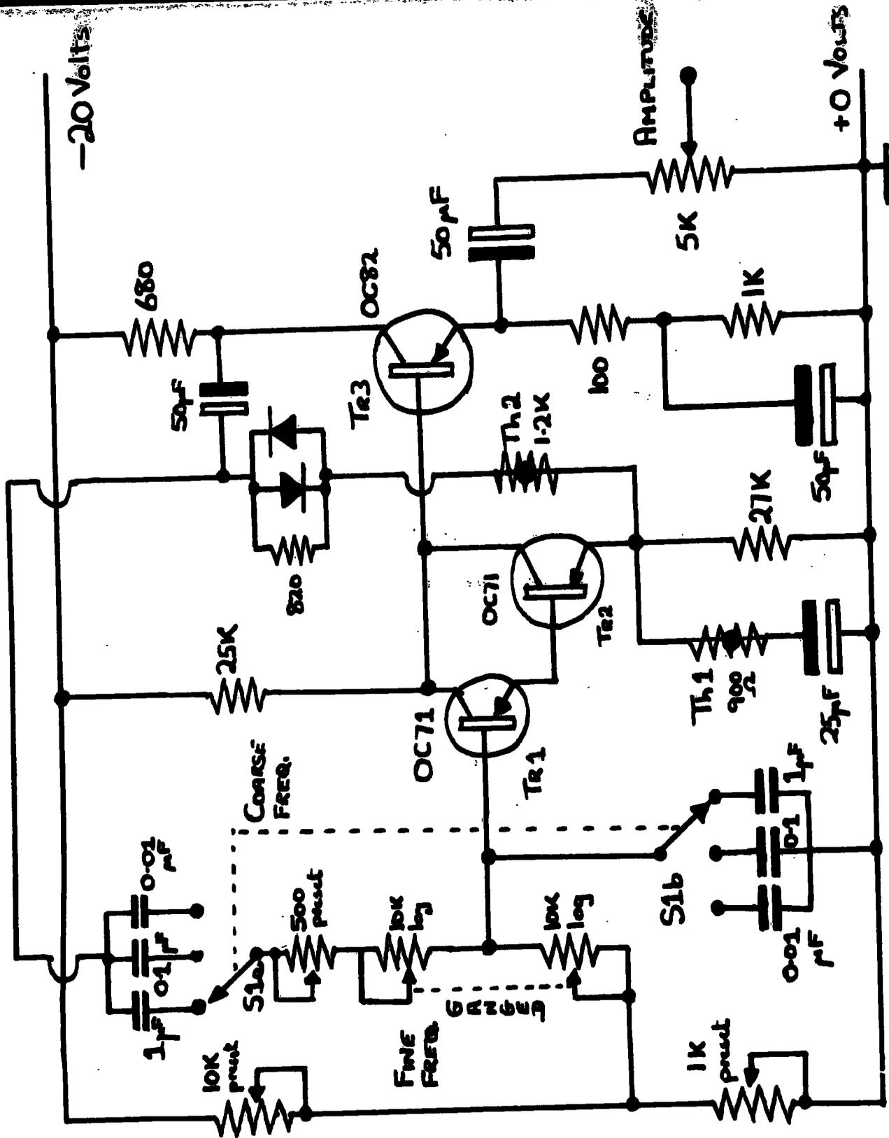
FIG. 4.3.2. WIEN BRIDGE OSCILLATOR CIRCUIT
