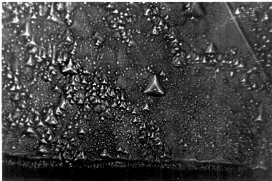
Figure (7.4) Etch pits on (111) cleaved plane of arsenic. The +ve y axis points from a pit centre normal to a pit side when the +Z axis is defined as the outward normal to the exposed cleavage plane.
