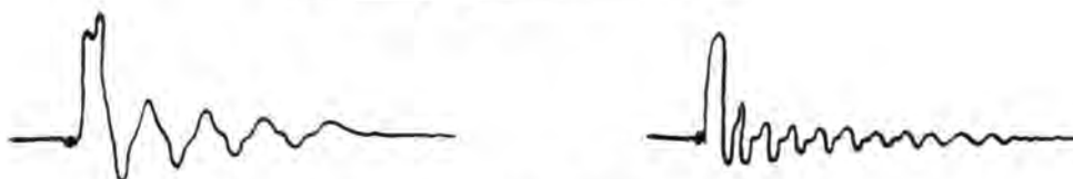
Fig. 51 . The nature of the repetitive pattern with R_t = 0 or \infty depends on the point of connection of the leads to the oscilloscope.
