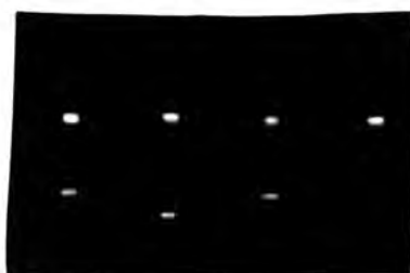
20.2 Tg 60, Ig 45, p 56, f 1.9. 8 trials; 8 sparks with multiple or diffuse channels.
