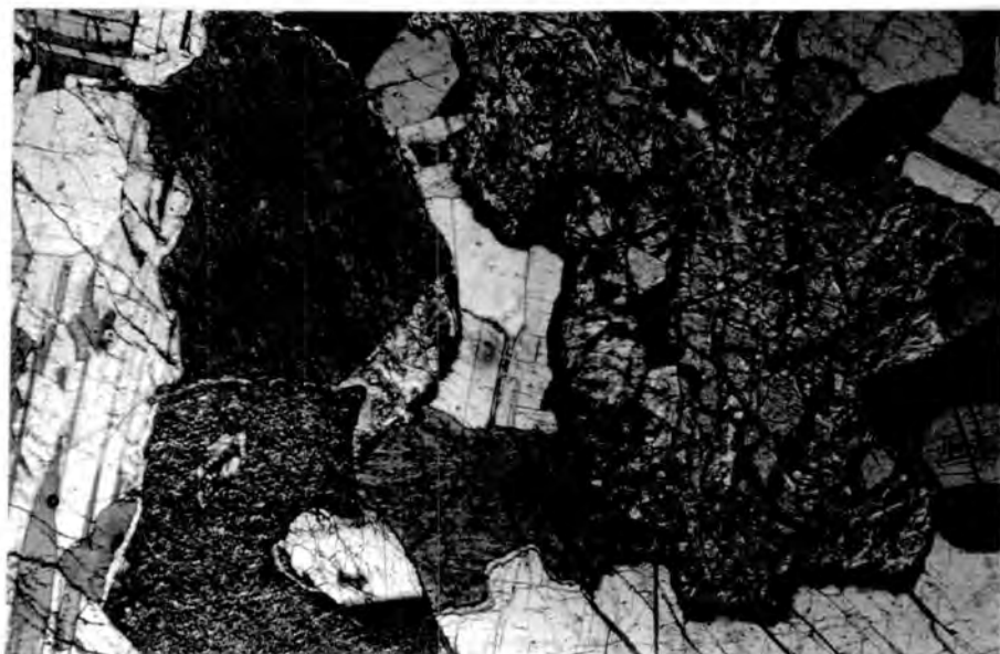
Fig. 67. Photomicrograph of olivine gabbro. T384 (crossed nicols X20). Notice the chlorite halo around the olivine.
