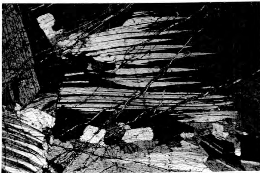
Fig. 70. Photomicrograph of feldspars in pyroxene gabbro. T331. (crossed nicols X50). Notice the pinched out lamellae.
