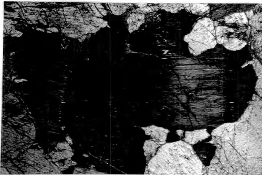
Fig. 39. Photomicrograph of kink band structure and clinopyroxene exsolution lamellae in orthopyroxene. T208 (crossed nicols X20).
