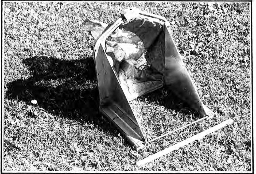
The net sampler : the rule in the foreground was 30cm. long.
