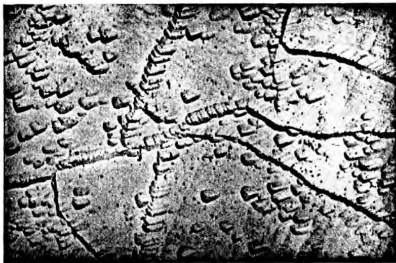
Figure 3. Etch pit pattern on (0001) face in central region of boule. Magnification \times 160 .
