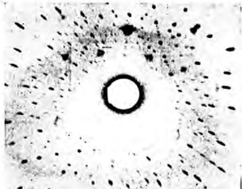
Figure 2. Specimen 1. Central region of ruby boule (concentration 0.35 \mu\text{g Cr per mg Al}_2\text{O}_3 ). Back reflection photograph taken 4.5 mm from boule outer surface. Beam parallel to c axis, \text{CuK}\alpha radiation.
