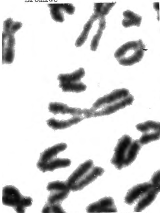
Fig. 61. 35 m.m. Microfile, developed in Microdol-X, printed on Grade 3 Bromide. Results most closely resemble those of the plate in terms of detail.
