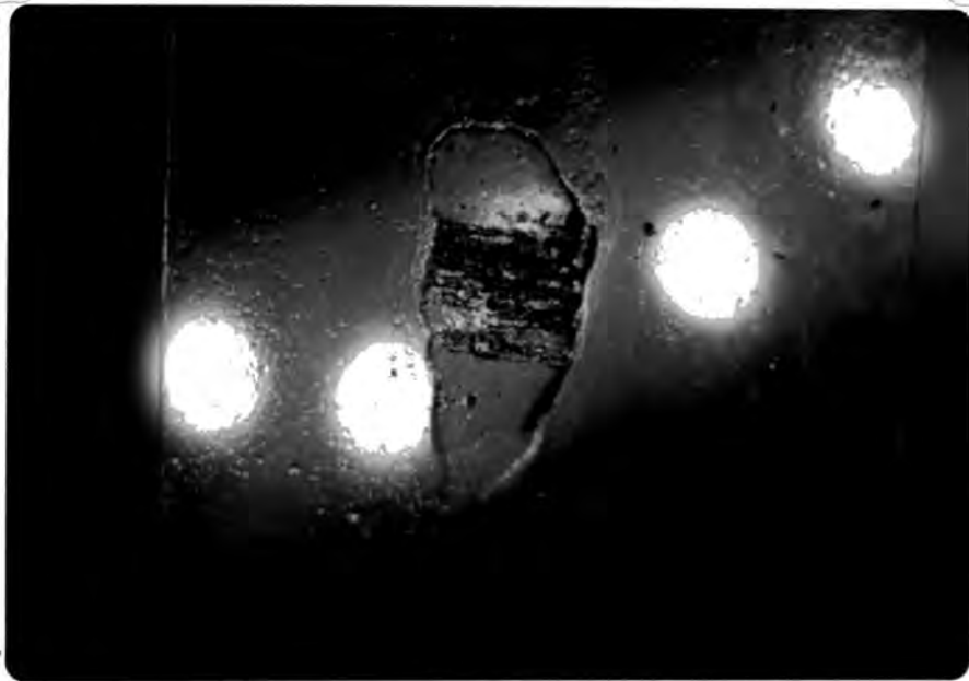
Fig. 70. Thin section of ice with dirt layer photographed in transmitted light.
