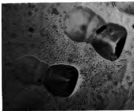
Figure 6. Etch pits produced from dislocations directed at an acute angle to the surface (etch A) ( \times 500 ).
