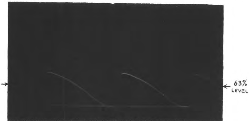
Fig. 10.6 (b) and (c) Oscillatory maintaining voltage oscillograms observed with hydrogen at 0.06 torr.
