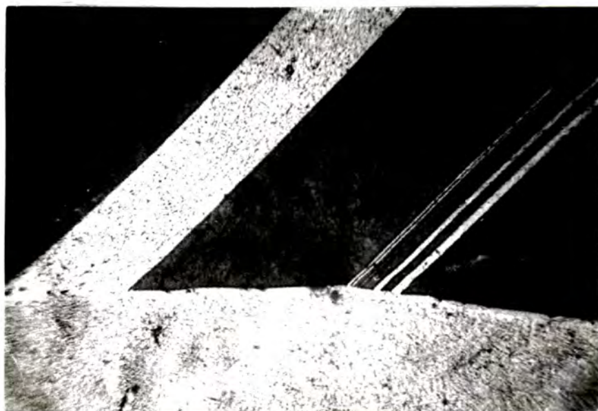
Fig. 3-3. Area of ZnSe Slice showing Twinned Regions and Grain Boundary. ( \times 200 )
