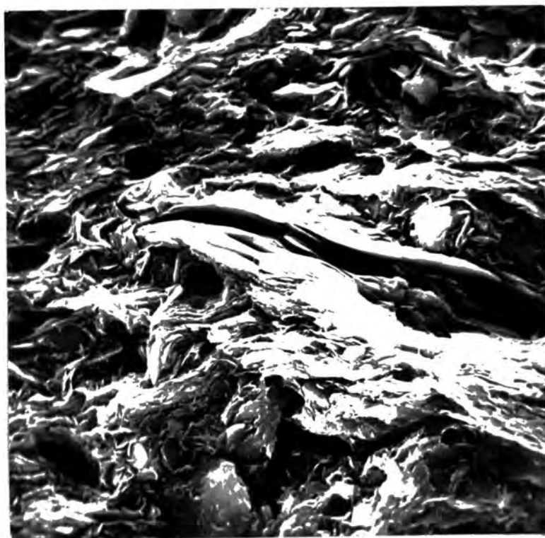
Figure 4.4. S.E.M. Photograph of London Clay 37m., x2400.
