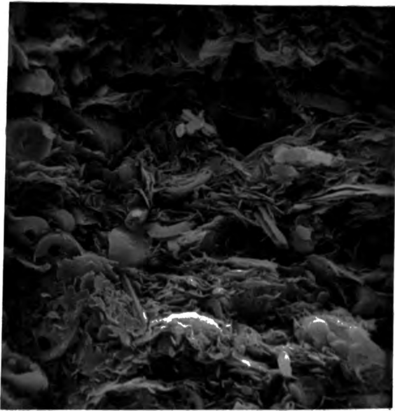
Figure 4.5. S.E.M. Photograph of Gault Clay, x2480.
