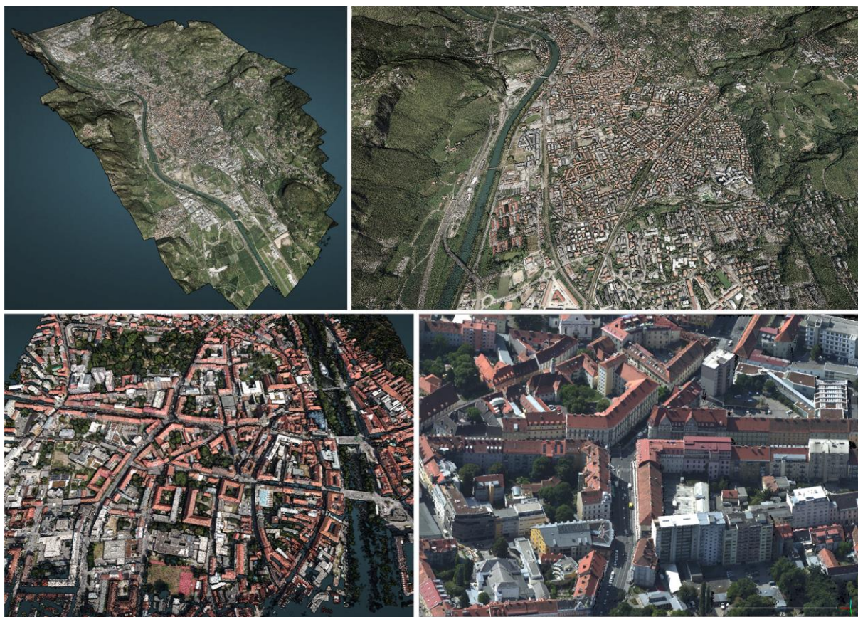
Figure 5. DSM cloud (5.5 billion points) of Trento (top) and 3D point cloud of Graz (bottom).
