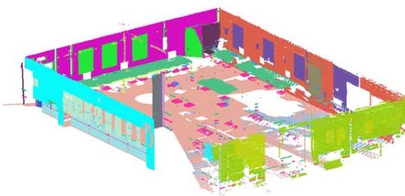
Figure 3: Extracted planes in the 3D space in an indoor environment (without the ceiling)
