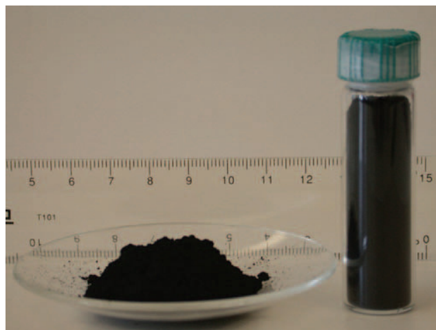
Figure 2.13. Example of the bulk quantity of graphene product. The image consists of approximately 2 g of sample. Picture taken from [66].
