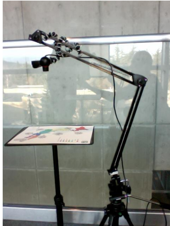
Figure 2: Shown above is a picture of the fiducial tracking interface. Above the computer monitor is a small consumer grade video camera, which is pointed downwards in order to view the fiducial markers which are placed on a printed paper map.
