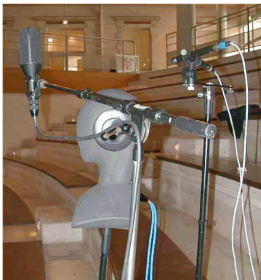
Figure 1. Simultaneous recording of the 3 techniques: artificial head for transaural reproduction, Soundfield microphone for ambisonics reproduction and ORTF pair for stereophony.
