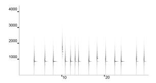
Figure 3: spectrogram taken from the virtual suikinkutsu. Frequency is represented on the y axis and time on the x axis.
