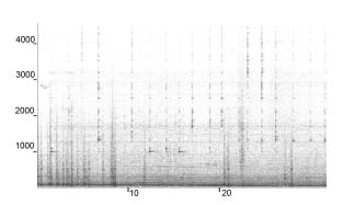
Figure 4: spectrogram taken from the physical suikinkutsu. Despite the large amount of background noise, droplets and the effect of the suikinkutsu body can be seen as vertical lines with modal peaks, which occur roughly once each second. Frequency is represented on the y axis and time on the x axis.
