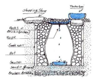
Figure 1: Cutaway of a suikinkutsu taken from [2].
