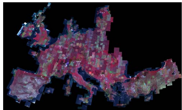
Figure 5 Example of orthorectified products derived from Spot 4 HRVIR, Spot 5 HRG and IRS-P6 Liss III data using automatically extracted GCP information from reference images for sensor model refinement. The overall geometric accuracy w.r.t. the reference is ~10m RMSE linear.
