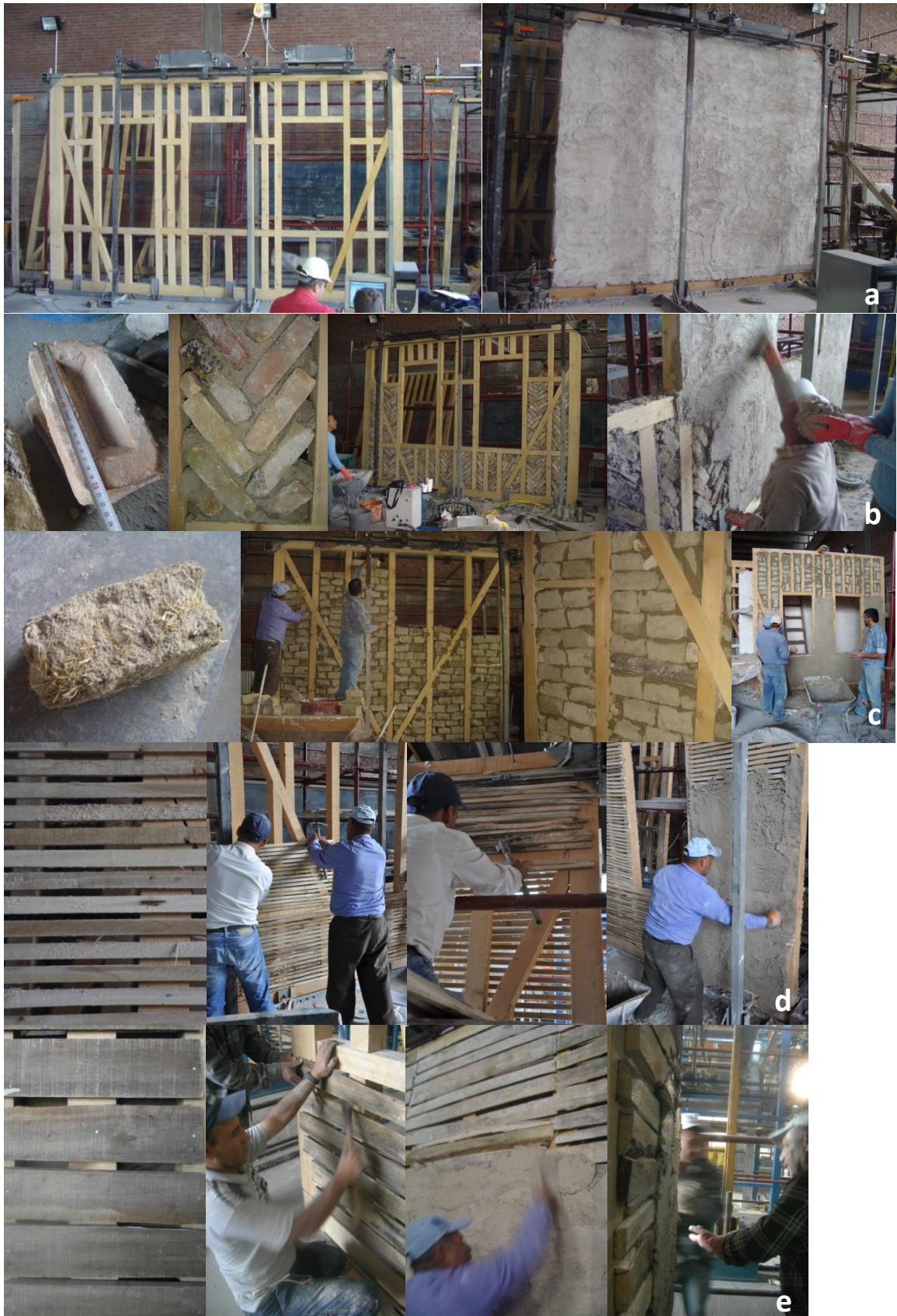
Figure 4: (a) Frame tests under reverse-cyclic lateral loading; (b) brick infill; (c) adobe infill; (d) bağdadi cladding; (e) şamdolma cladding.
