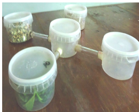
Fig. 1 Four arm choice chamber consist of four transparent plastic containers
