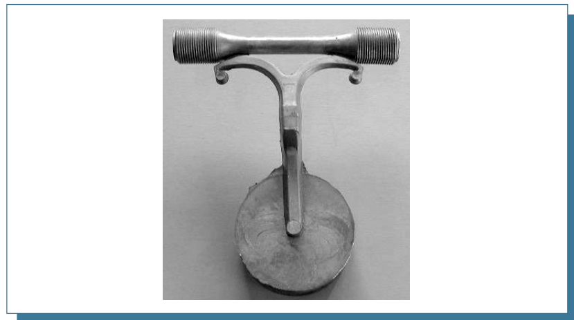
Fig. 2: Sprue-runner design for high porosity range (A4)
