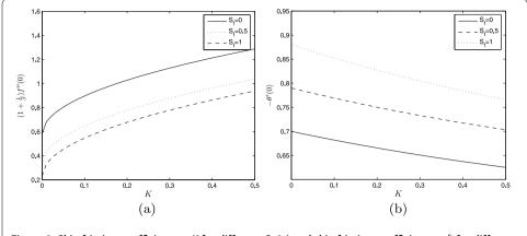
Figure 8 Skin friction coefficient vs. K for different  $S_f$  (a) and skin friction coefficient vs.  $\xi$  for different  $S_T$  (b) at  $\beta = 2$ ,  $\Lambda_1 = 0.5$ , M = 1, Pr = 1, Ec = 1,  $f_W = 0.5$ ,  $\Lambda = 0.5$ .
