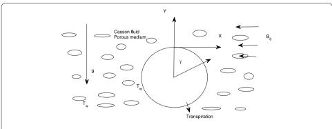
Figure 1 Schematic of the problem circle in a Casson fluid with transpiration.
