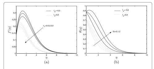
Figure 5 Effects of  $\Lambda_1$  and Ec on (a) velocity and (b) temperature profiles for different  $f_w$ , at  $\beta=2$ ,  $\Lambda=0.5$ , K=0.5, M=1, K=0.5, Pr=1,  $S_T=0.5$ .
