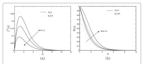
Figure 3 Effects of magnetic parameter on (a) velocity and (b) temperature profiles for different  $S_f$  and  $S_T$ , at  $\Lambda_1=0.5$ , K=0.5, F=1, E=1, F=1, F=
