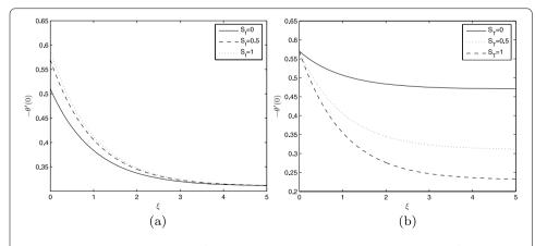
Figure 7 Heat transfer coefficient vs.  $\xi$  for different  $S_f$  (a) and skin friction coefficient vs.  $\xi$  for different  $S_T$  (b) at  $\beta=2$ ,  $\Lambda_1=0.5$ , K=0.5, M=1, Pr=1, Ec=1,  $f_w=0.5$ ,  $\Lambda=0.5$ .
