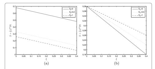
Figure 6 Skin friction coefficient vs.  $\xi$  for different  $S_f$  (a) and skin friction coefficient vs.  $\xi$  for different  $S_T$  (b) at  $\beta=2$ ,  $\Lambda_1=0.5$ , K=0.5, M=1, Pr=1, Ec=1,  $F_w=0.5$ ,  $\Lambda=0.5$ .
