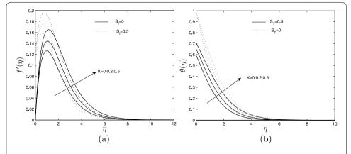
Figure 4 Effects of radiation parameter on (a) velocity and (b) temperature profiles for different  $S_f$  and  $S_T$ , at  $\beta=2$ ,  $\Lambda_1=0.5$ , K=0.5, F=1, F
