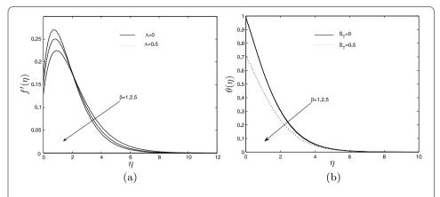
Figure 2 Effects of Casson parameter on (a) velocity and (b) temperature profiles for different  $\Lambda$  and  $S_T$ , at  $\Lambda_1=0.5$ , K=0.5, P=1, E=1, E=1,
