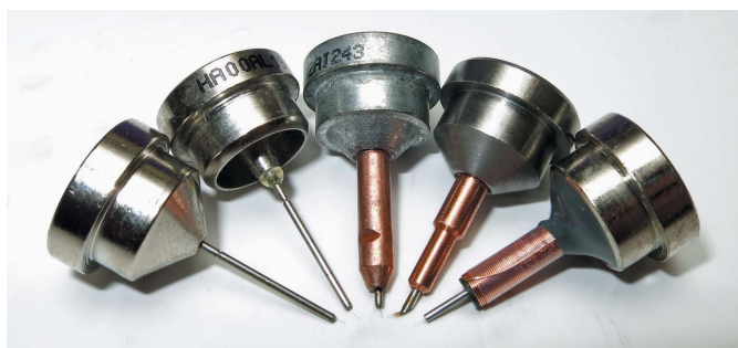
Figure 4 Close-up of five cryomounts. Left to right: Hampton Research ALS-style with steel pin; SPINE with steel pin; Hampton Research CryoCap copper with ledge; MiTeGen copper RT; Rigaku RFID mounting pin.
