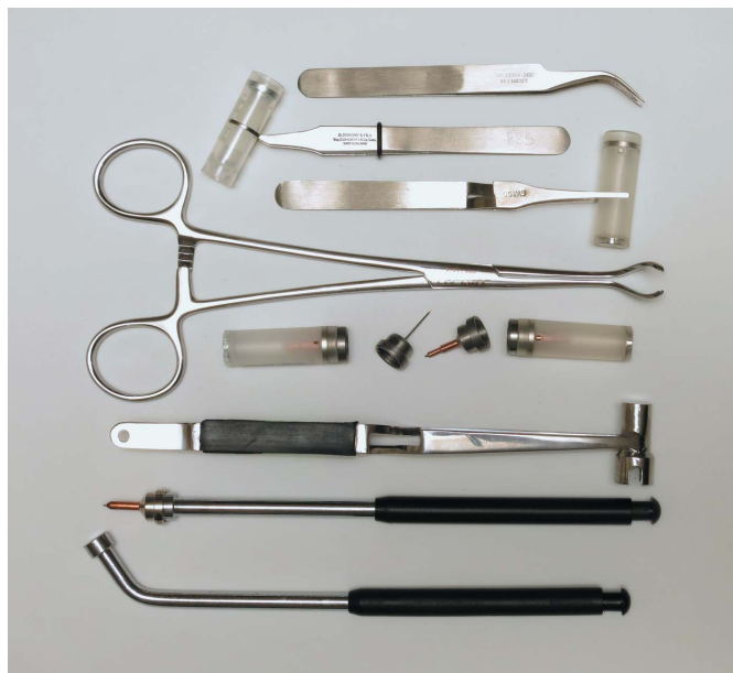
Figure 3 Hand tools for cryocrystallography. From the top: forceps for grasping mounting pins; cryovial forceps with O-ring to maintain closure; self-closing forceps to hold vials and mounts without finger pressure; cryovial locking tongs; cryovials and cryobases with pins and loops; cryotongs; straight magnetic wand; curved magnetic wand. Items are from Hampton Research, MiTeGen and Molecular Dimensions
