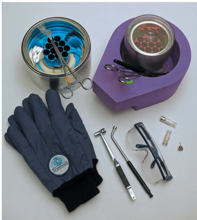
Figure 2 Accessories for cryocrystallography. Clockwise from lower left: gloves; shallow Dewar with automounter puck and clamping tongs holding a cryovial; purple foam Dewar holding a small glass Dewar with clear plastic cover; cryovials, cryomounting pin; safety glasses; curved magnetic wand; cryotongs.
