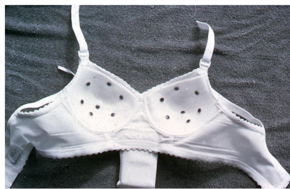
Figure 1 The Chronobra: a custom built thermometric brassiere with 16 channel automated electronic thermometry for measurement of the heat cycle in the breast.
