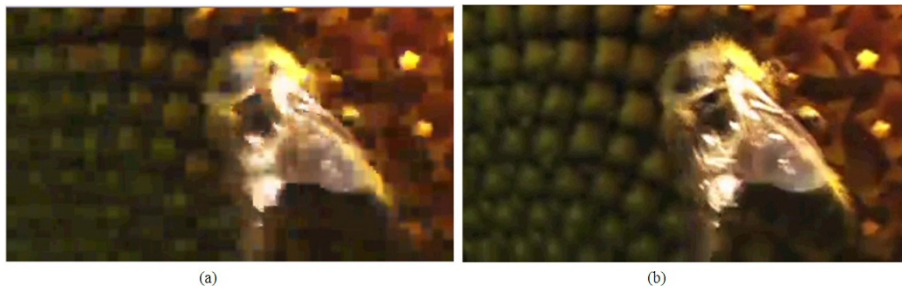
Figure 7 76th frame image of Sunflower sequence with 600 kbps: (a) conventional rate control, (b) proposed rate control.
