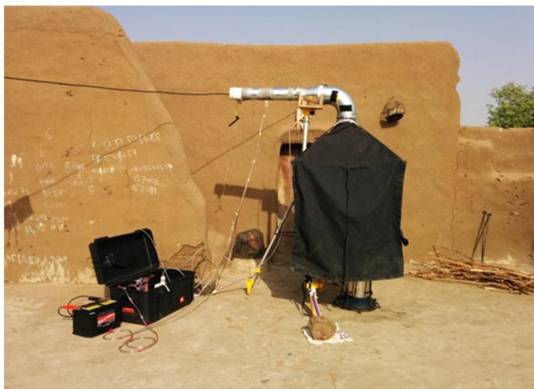
Figure 5 E-Pod setup for measuring in-field stove emissions.
