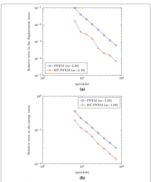
**Fig. 5** Bending of thick cantilever beam: convergence results for **a** the relative error in the displacement norm ( $L^2$ ) and **b** the relative error in the energy norm. The rate of convergence is also shown, where m is the average slope. In case of the polygonal SBFEM, p denotes the order of the shape functions along each edge of the polygon
