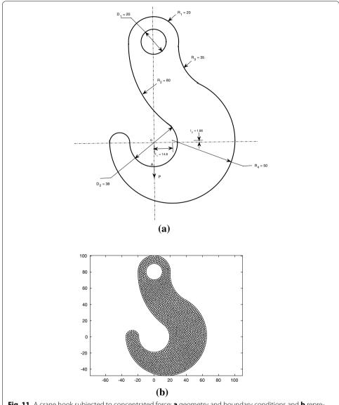
**Fig. 11** A crane hook subjected to concentrated force: **a** geometry and boundary conditions and **b** representative mesh
