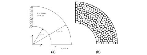
**Fig. 8** Geometry, boundary conditions, and representative polygonal mesh for a curved cantilever circular beam. The displacements at the left end are constrained and a constant displacement is applied at the other end
