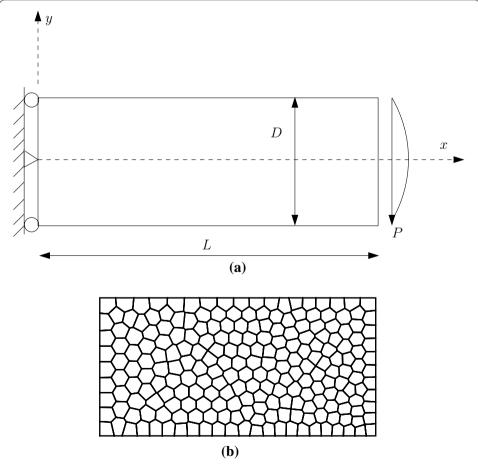
**Fig. 4** Cantilever beam: **a** geometry and boundary conditions and **b** representative polygonal mesh. The domain is discretized with 100 elements
