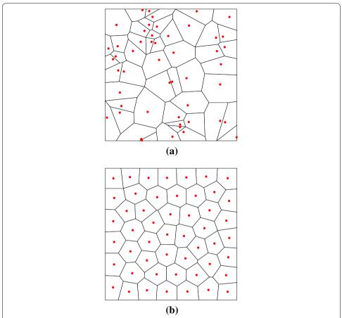
**Fig. 2** Voronoï tessellation, where the *red dots* are the seed points: **a** scattered dataset; **b** polygonal mesh after few iterations
