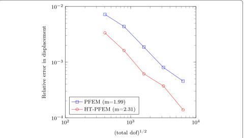
**Fig. 7** Infinite plate with a circular hole: convergence results for the relative error in the displacement norm  $(L^2)$ . The rate of convergence is also shown, where m is the average slope
