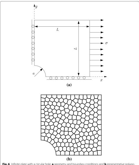
**Fig. 6** Infinite plate with a circular hole: **a** geometry and boundary conditions and **b** representative polygonal mesh
