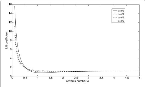
Figure 3 Lift coefficient versus Alfvén's number. The lift coefficient is calculated for various values of the angle  $\alpha$ .
