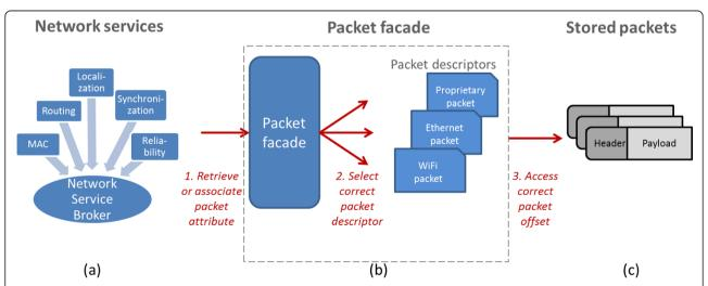
**Figure 3 Network services can transparently interact with any packet type. a** Network services can associate metadata with, or retrieve metadata from, stored packets using the packet facade. **b** Only the packet facade requires knowledge about the packet format. As long as the correct packet descriptor is available, the packet facade knows how and where metadata is stored. **c** Finally, the packet facade accesses the correct header offset or the packet payload.
