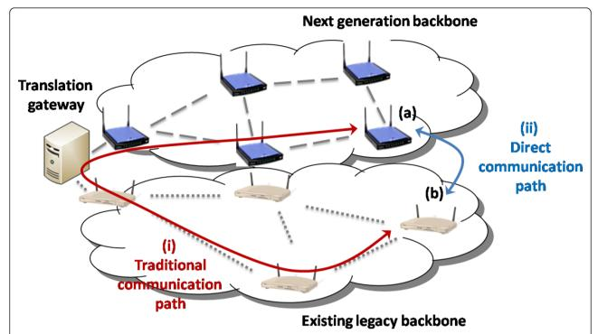
**Figure 4** The coverage of an existing legacy network is expanded by installing an additional next-generation backbone. (*i*) Using existing technology, all communication must pass through a translation gateway, resulting in suboptimal use of the network. (*ii*) A next-generation IDRA network can converge with existing networks and use direct communication paths, thus prolonging the operational lifetime of legacy networks.
