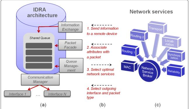
**Figure 2 Conceptual presentation of the IDRA architecture. a** The IDRA system is responsible for packet creation, packet storing and packet interactions. **b** Interactions between the network services and IDRA are mainly descriptive in nature. **c** Network services can be added dynamically according to the needs of the device.
