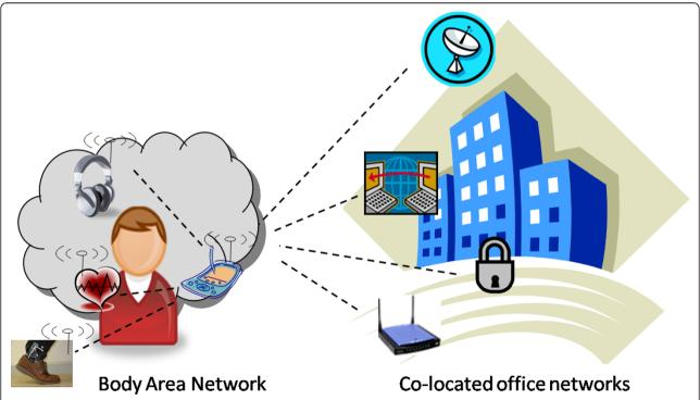
**Figure 5** A resource-constrained personal Body Area Network (*BAN*) monitors the health of an employee. For efficient communication, the BAN should be able to communicate directly with all co-located network technology such as wireless entrance and security control, UMTS, Wi-Fi and DECT.
