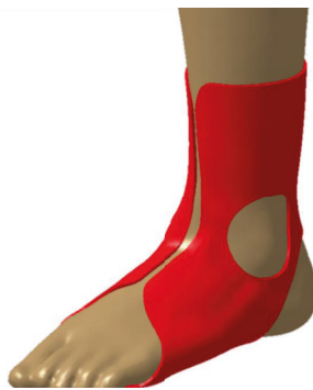
FIGURE 4: Using the adjustment of the joint axis, the 3D modelling of individualized AFO with correction of the axis was designed.
