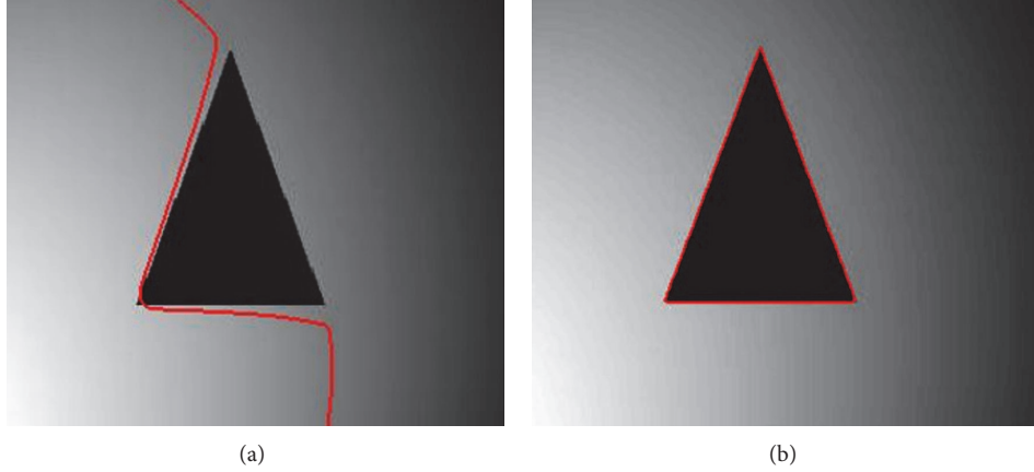
FIGURE 1: Intensity inhomogeneous image segmentation using global and local intensity based active contour methods. (a) Segmentation result using Chan-Vese method. (b) Segmentation result using LBF method.
