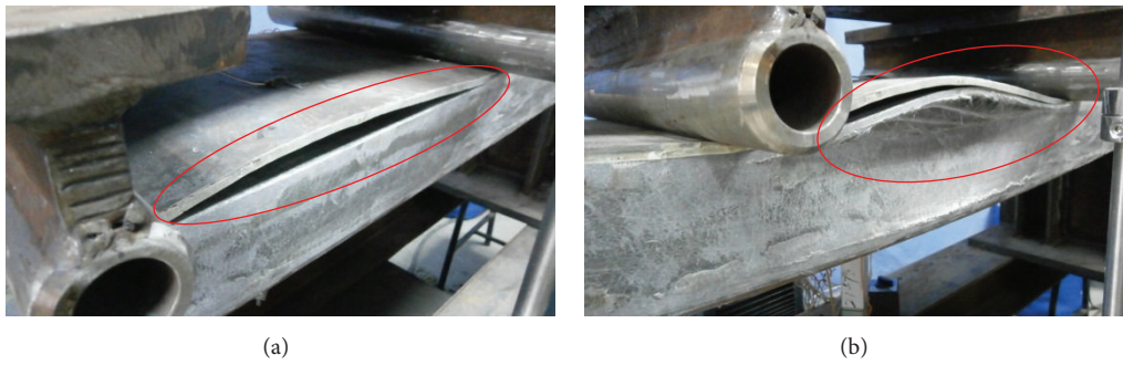
FIGURE 5: Failure of specimen S(4)-GFRP: (a) peeling off and delaminating and (b) tearing failure of the web where it intersected the facesheet.
