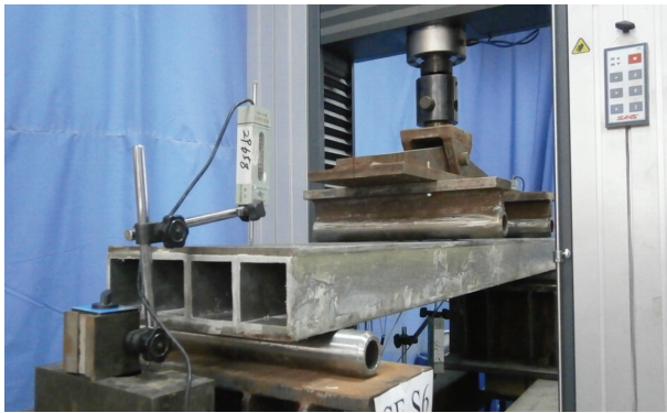
FIGURE 3: Flexural test setup.
