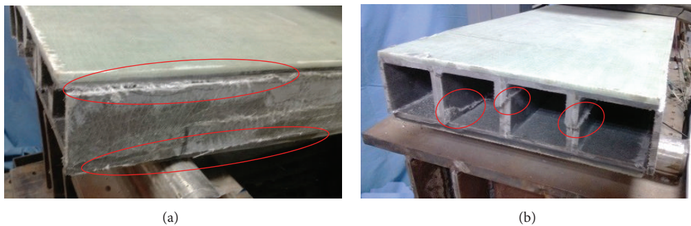
FIGURE 9: Failure of specimen F(6)-GFRP: (a) cracks spreading horizontally and (b) rib fracture.
