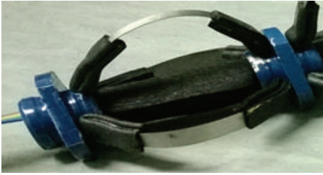
FIGURE 10: Prototype of the EAP-based flexible actuator.
