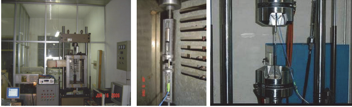
FIGURE 18: Fatigue test of FRP-packaged FBG strain sensor.
