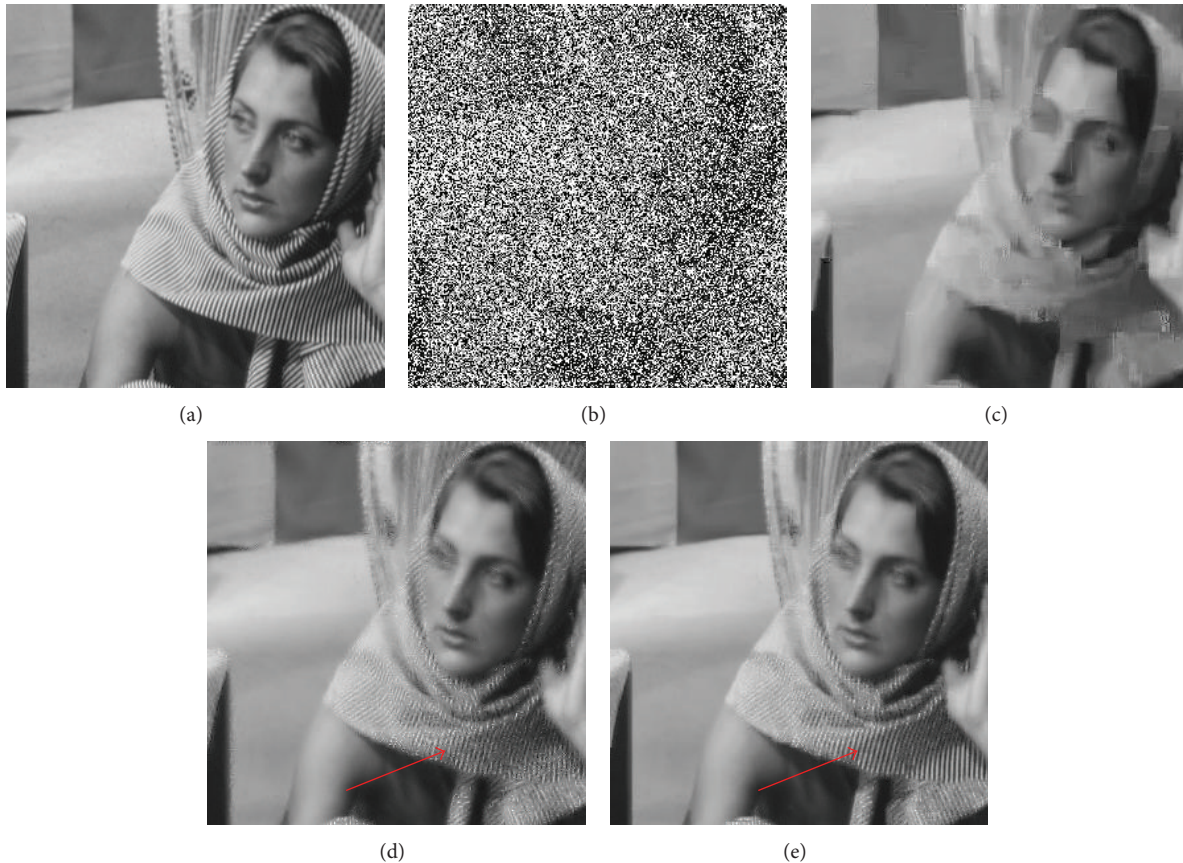
FIGURE 12: Denoising results of Barbara image with 70% salt-and-pepper noise. (a) Ground truth image, (b) noisy image, and (c), (d), and (e) are denoised images using the proposed method, total variation with noise detectors, and the proposed method with noise detectors, respectively.
