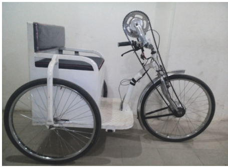
FIGURE 5: The developed electrically assisted wheelchair incorporated with a torque sensor pedal.
