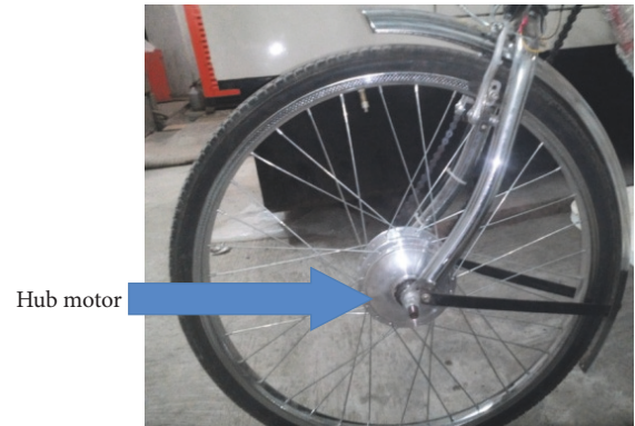
FIGURE 7: A 250 W hub motor attached to the front wheel.
