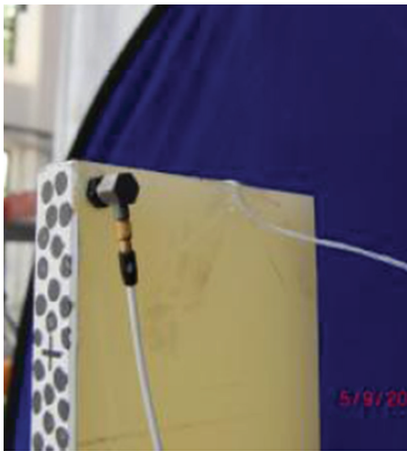
FIGURE 5: Installed accelerometer at the end of tested sample.
