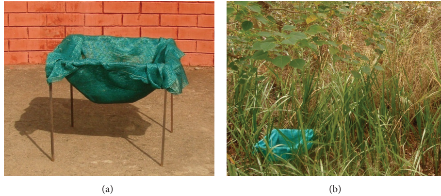
FIGURE 1: (a) Litter trap of dimension 50 \times 50 \times 50 \text{ cm}^3 and (b) its placement in the site.
