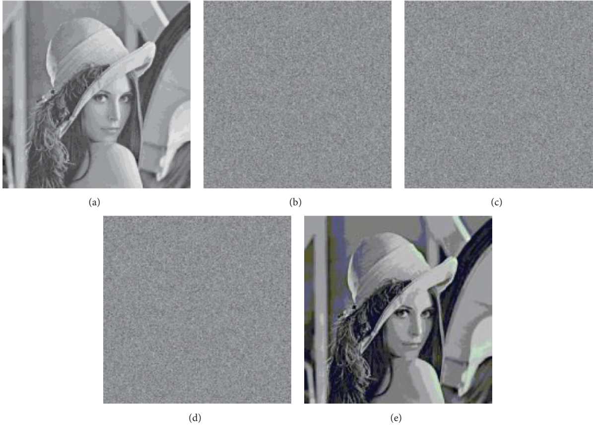
FIGURE 2: (a) Original image; (b) encrypted image; (c) encrypted image containing watermark; (d) reconstructed image; (e) decrypted image.
