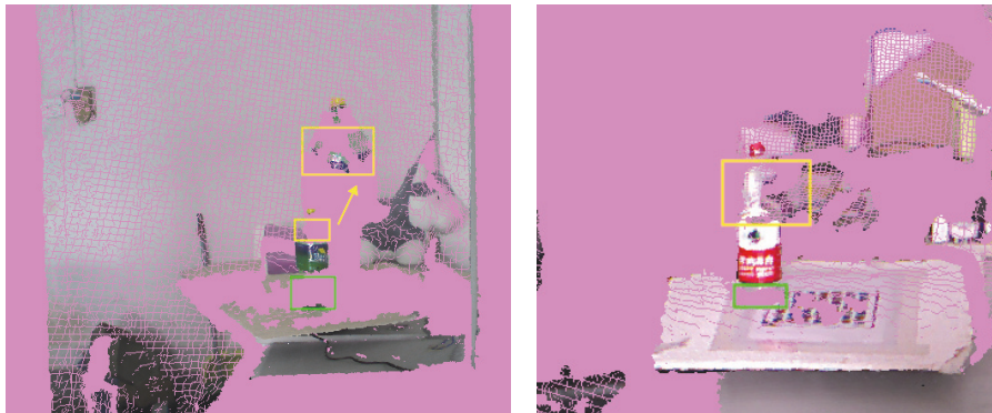
FIGURE 3: 3D point clouds show two kinds of depth appearance of transparent object; Green rectangles label the zero-depth noise which is consistent across frames. Yellow rectangles label the wrong depth noise mingled with zero depth which keeps on changing across frames; the wrong depth may be drifted to a farther location than the real value.
