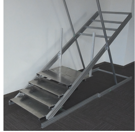
FIGURE 17: Changeable mockup stairs.
